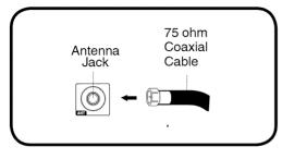
For basic Cable TV service not requiring a Converter/ Descrambler box, connect the 75 ohm Coaxial Cable directly to the Antenna Jack on the back of the TV.
